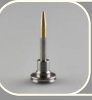
The piston bullet for Atomic first stage helps slide the piston assembly during the Atomic Aquatics regulator service through the first stage body while protecting the critical knife edge and preventing the o-ring from damage.
