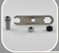
During the frequent use of this tool in our own service center, we have noticed that the splines in the aluminum and plastic version of this tool wear slowly and therefore no longer fit perfectly around the hose nut. To solve this problem, we redesigned the tool in a 304 stainless steel finish
