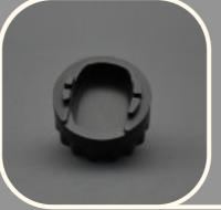
The Mares Fusion cover tool is used to open the cover of the Mares Fusion second stage by sliding it over and locking the four tips into the recesses of the second stage cover.
